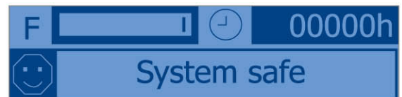
Filter Life Indicator (For Type A2 Motorized-control & Type B2 Models)
